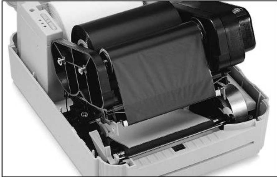
Figure 10. Installation of label stock and thermal transfer ribbon
