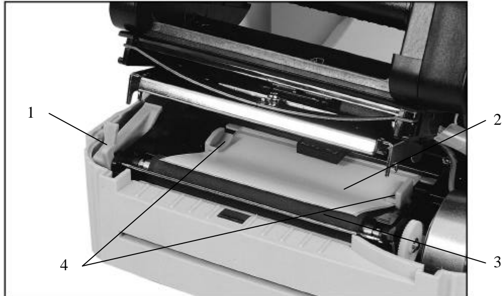
Figure 6. Feed labels through adjustable label guide
